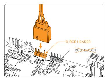
Plug the 3-pin connector of the Wire Harness to the D-RGB HEADER on the motherboard. The LED will work if the pin layout on the header is as follows: **+5V, Digital, Empty, Ground**.
