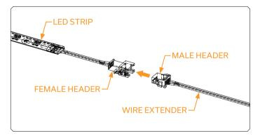
The EK-Loop D-RGB LED Magnetic strip contains 21 LEDs and 500 mm wire harness. The wire extenders (150 mm) allow you to connect more LED strips to customize your PC LED lighting (shown in the image).
