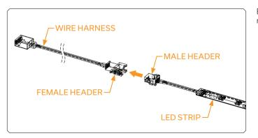
Before connecting the LED strip with the motherboard, Wire harness must be attached as shown in the image.
