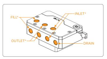
EK-Quantum Kinetic FLT has two inlet and two outlet ports, one of each must be used!
