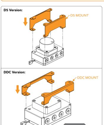
To enable installation of the reservoir where clearance for the pump is required, EK supplies a pair of FLT mounts along with M4 nuts, washers and additional screws.
