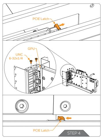
Before you mount the GPU, make sure the PCIE latch is not closed – it must be pushed to the right side.
