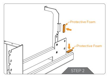
Stick two protective adhesive foams, as indicated in the diagram. The »2mm protective foam« should be enough for the protection of your GPU during installation. In some cases, you may use the »5mm protective foam« (also enclosed in the package) for the extra support of your GPU.
