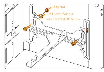
EK-Loop Angled Bracket can be mount directly into the case when there is a place for a 120mm fan.
