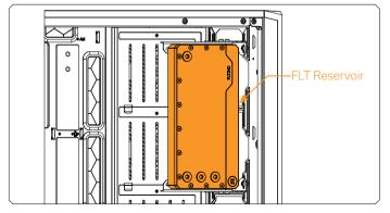
After securing the EK-Loop Angled Bracket into the chassis, you can attach the FLT reservoir. (See chapter: **Attaching the FLT Reservoir to the EK-Loop Angled Bracket**)
