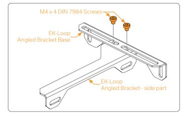
For the assembly of the EK-Loop Angled Bracket, use M4 X 4 DIN 7984 screws (as shown in the picture). Side parts already have threaded holes, so there is no need for additional washers and nuts.
