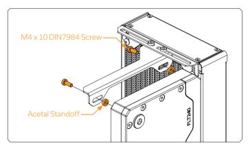
Carefully position the FLT reservoir onto the EK-Loop angled bracket and secure it with the enclosed M4 X 10 DIN 7984 screws and acetal standoffs (as shown in the picture). While tightening the screws, do not use excessive force. Make sure that all four (4) screws and standoffs are adequately secured!
