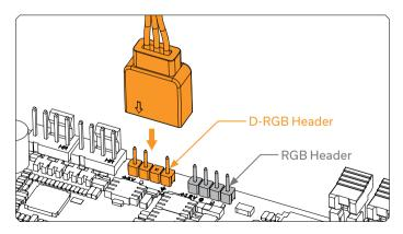
Plug the 3-pin connector from Water block's D-RGB LED light to the DRGB HEADER on the motherboard. The LED will work if the pin layout on the header is as follows: +5V, Digital, empty, Ground.
