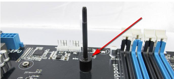
3. Screw the posts into each of the four holes around the socket.
