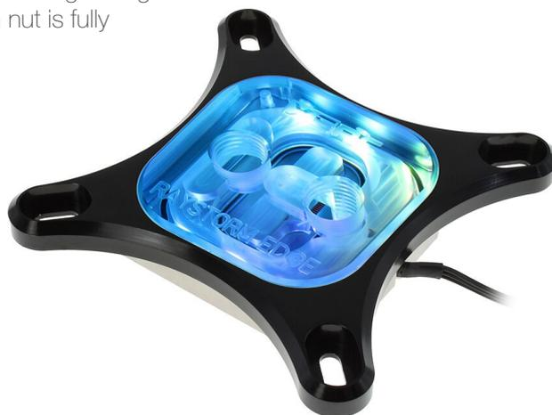
7. The block is now ready to use. When you first boot it is advisable to use software to check the core temperature. If the temperature is high you will need to remount the block.
