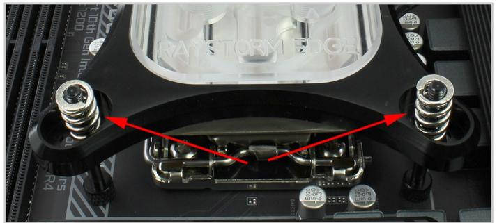
4. Place a spring over each of the four posts and into the wells on the hold down bracket.
