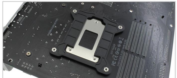
2. Make sure the 4 screw threads on the backplate line up with the holes on the motherboard. Apply pressure to secure the backplate.
