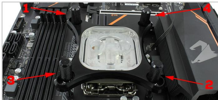
5. Place a nut onto each post and gradually tighten them. You should tighten each nut in stages. e.g. 1,2,3,4,1,2,3,4,1,2,3,4, until each nut is fully tightened.
