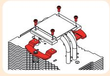
Then fix the new NM-IFB2 fastening brackets to the cooler (you can either use the original screws or the supplied NM-SSC1 screws).
