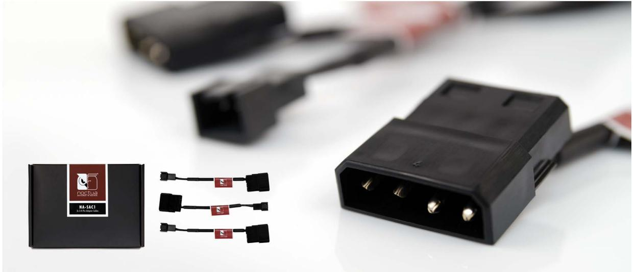
The NA-SAC1 is a fan accessory set consisting of three fully sleeved NA-AC1 3:4-Pin Adaptor Cables. The NA-SAC1 adaptors allow connecting standard 3-pin fans to the power supply's 4-pin peripheral connectors. Thanks to the loop-through design of the 4-pin connector, you can still connect other devices or further adaptors.
